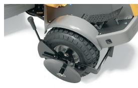
5. Rezalnik robov 2WD+4WD
